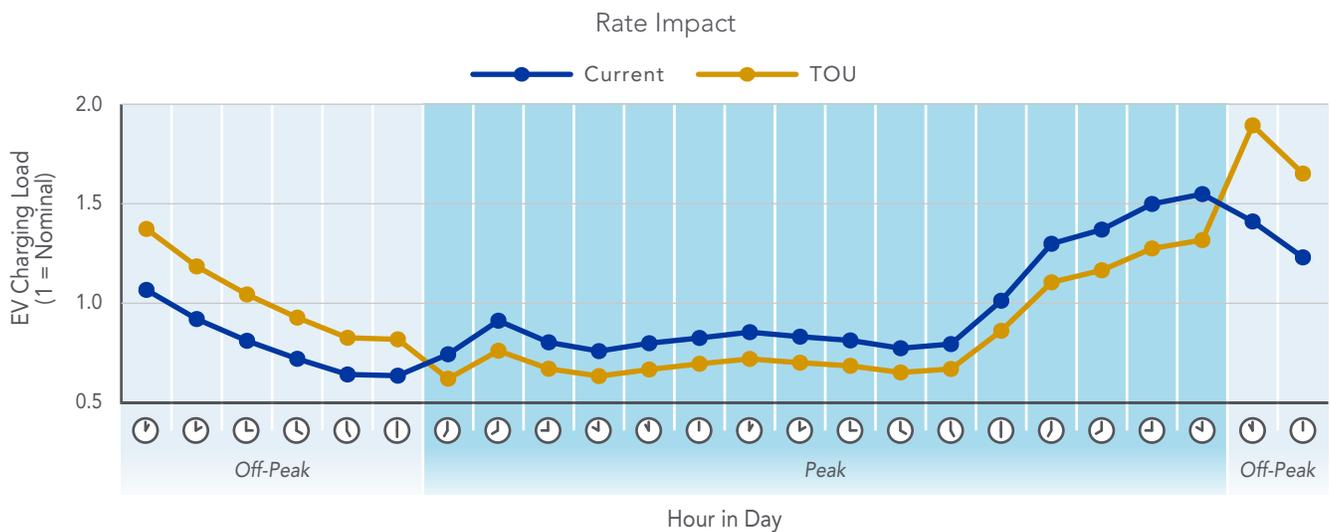
As the figure indicates, the new rate is projected to encourage a shift of only a modest fraction (less than 20%) of the EV charging load into the off peak period. The best the utility can do with a two-part TOU rate under these conditions is to provide EV buyers with a savings of \$50/year. This is a very small fraction of their total utility bill and their annual EV operating cost.
