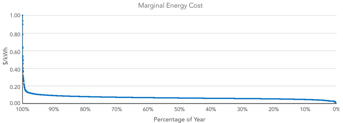
A big part of the reason for the relatively small change in behavior is that the rate structure does a poor job of reflecting real costs. Using real but disguised data, the figure above shows the variation in marginal energy costs to the utility over the 8760 hours in a year.
